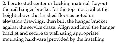
contractor using wood screws, toggle bolts, sheet metal screws, etc. as per local code].
