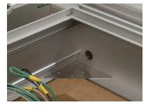
extrusion, but not the plastic laminate on the outside. Use a screwdriver or utility knife to punch out the plastic. Insert the plastic bushing that is provided with the light fixture into the hole, mount the light fixture and feed the three wires from the light fixture through the hole and connect to the three taped wires provided. [Wire connectors are provided]
