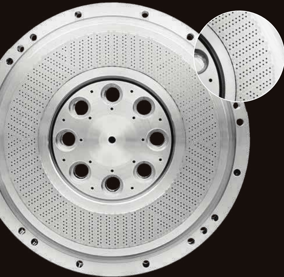
For Berstorff underwater Pelletizer UWG 50 with 1160 holes Heat Channel design, steam heated
