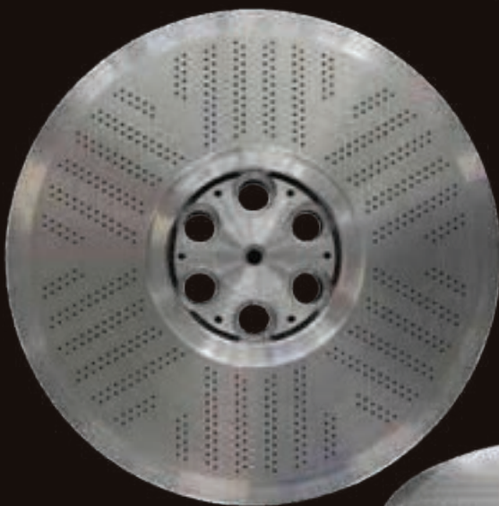
Steam heated Die Plate, Heat Channel design for LDPE with 696 holes
