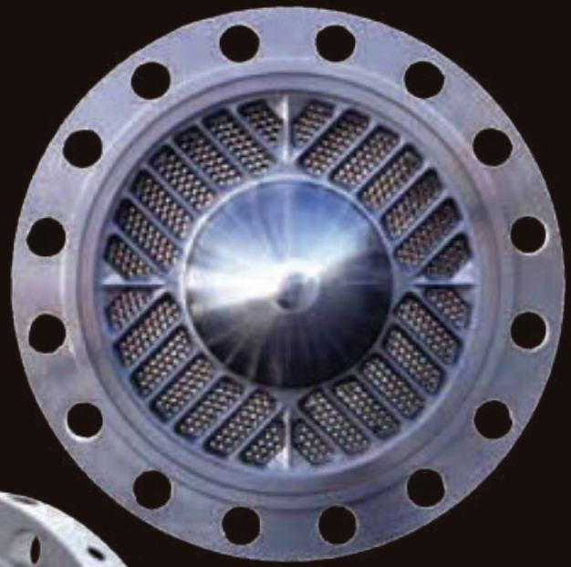
For Farrel underwater Pelletizer S. 1200 with 532 holes Heat Channel design, steam heated
