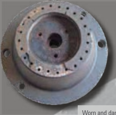
Worn and damaged Gala Die Plate before reconditioning
