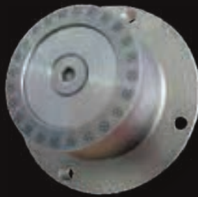
Die Plate for Micropellets with 360 holes x 0,65 mm diameter
