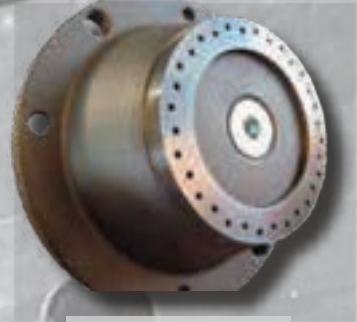
Die Plate after replating with TiC segments
