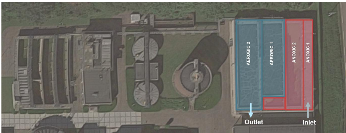
Figure 1: Layout and configuration of the industrial wastewater treatment plant under investigation. The wastewater has municipal characteristics but is highly dynamic and has a rather high ammonia load.
