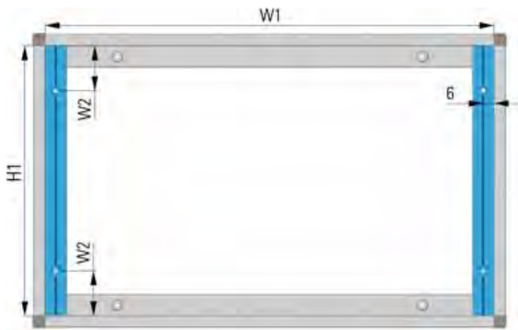
Rear view for cases made of frame extrusions with depth D1 = 130 mm
