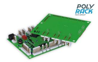
The new system monitoring board SMC3 from POLYRACK has a size of only 80 x 75mm and monitors and controls up to six fans divided into three groups.
