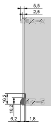
Side view, bottom-hinged / side-hinged with hinge extrusion
