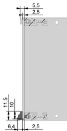
Side view, bottom-hinged / side-hinged with hinge element
