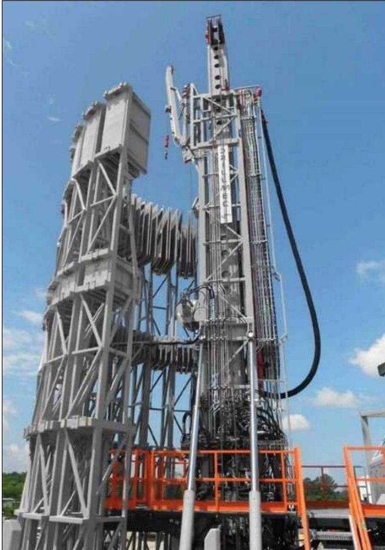
Figure 3.4-1 Example Drill Rig for a Slim-hole Well
