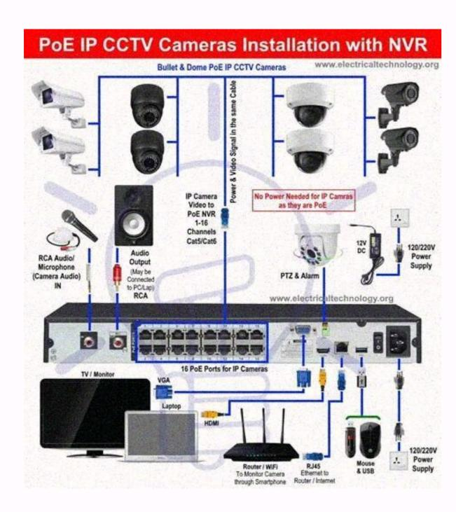
To set up an IP camera network, you need to deal with two main tasks: setting up the cameras to send data out and setting up your devices to receive data locally and remotely. We'll break this down into two parts (Part 2 and Part 3) for easier understanding. Attention: Not all phone or PC access to IP cameras is remote viewing. The type of viewing depends on whether you access the camera in LAN or WAN.
