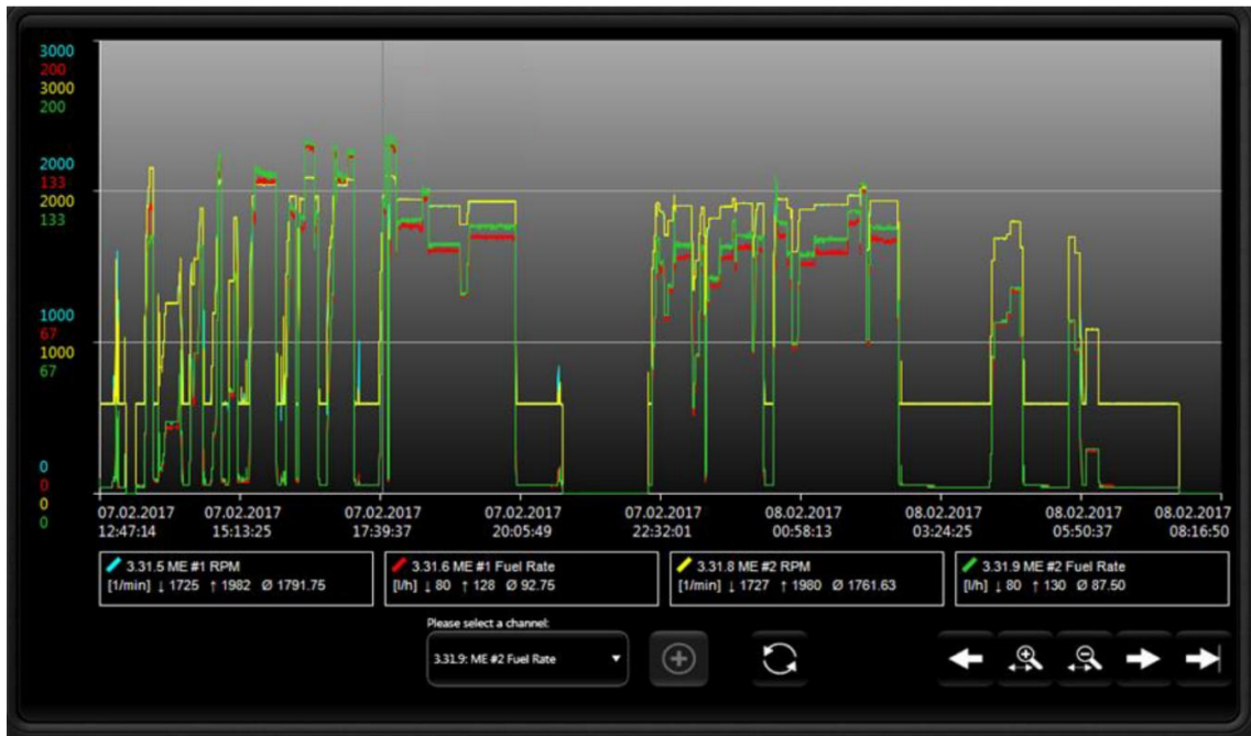
Figure 3: Data logging / trending page with multiple graphs (up to 8 measurement channels possible)
