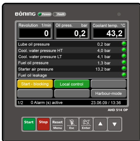
Illustration 48: "Start – blocking" after activating "system off"
