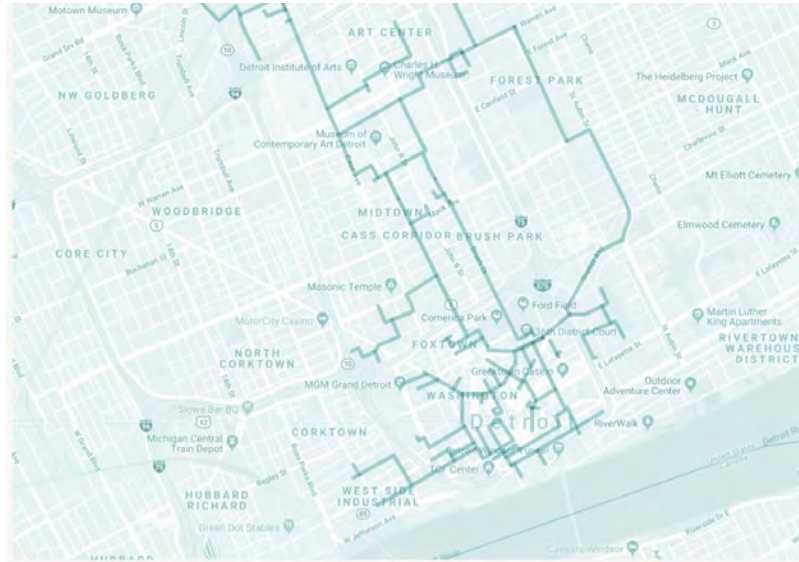
Map of Detroit Thermal's underground steam distribution loop in downtown Detroit
