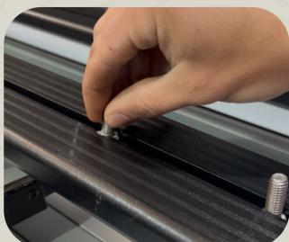
**3.** Using the 4x (four) Load Bar Mounting brackets, remove the 2x (two) hex bolts from the bottom of the bracket. Slide the 2x (two) hex heads into the load bar on the roof rack.
