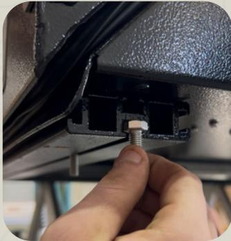
**6. Prepare the tent:** Remove the hex bolt from the top of the Load Bar Mounting Brackets. Slide it into the center slot of the load bar underneath the Nyumba (2x (two) Hex heads in each load bar).
