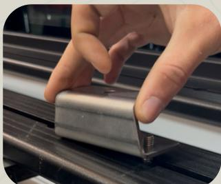
**4.** Place the Load Bar Mounting brackets onto the bolts and loosely tighten. (Repeat with the 3 remaining brackets)
