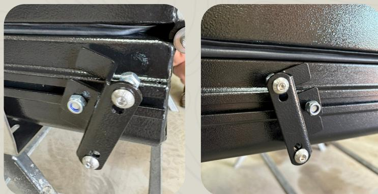
**3. Measure** the distance between the shower's mounting holes. Adjust the brackets to match this distance, then tighten them securely.
