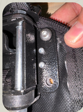
Step 3: Inserting of bolts in mounting holes
