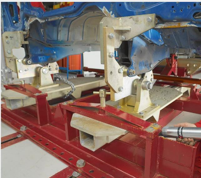
The four mounting points of the damaged cab are anchored to the bench by means of specially designed adapter sets for each cab model. Badly displaced front mounting points are held and pressed into the correct position by using a hydraulic cylinder and moveable jig members.
