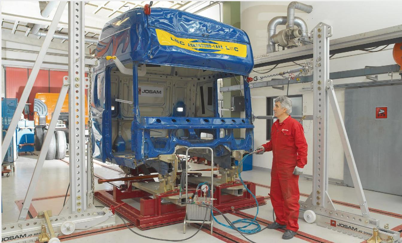
**The JOSAM cab bench is a strong and stable aligning jig which simplifies cab repair. Moveable mounting points make it easier to mount even severely damaged cabs.**
