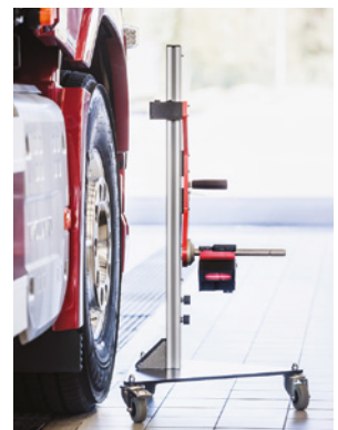
Touchless chassis and body sensing tool
