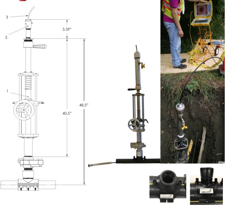
Example Application: 2" IPS Pipe Dimensions Shown With Tool Fully Retracted
