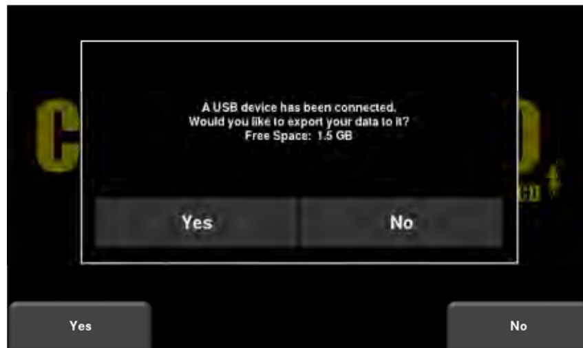
Figure 11-2: When a USB drive is connected to the Display Unit, a message opens asking if you would like to export all your data to it. Select Yes to transfer immediately. If you select No , you can export the data later by going to the Setup > File Management menu option.
