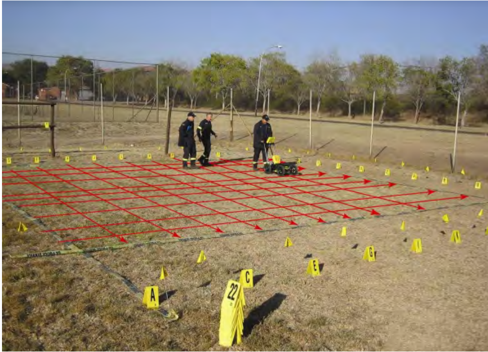
Figure 7-2: Example of a grid survey. The red lines are superimposed just to illustrate the concepts.
