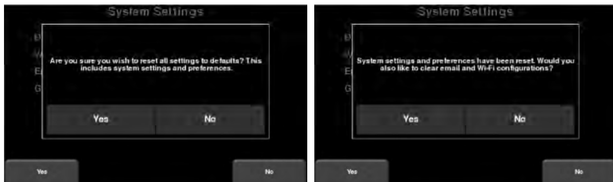
Figure 4-5: Reset to Defaults, a) Image on left is the first confirmation screen. b) If you press Yes, you will see the second confirmation screen on the right asking about deleting e-mails and WiFi settings.
