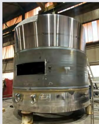
Right: Preassembly of the Main drive in the final state. Left: Machining of the shield finished and welding of the Lifting lugs
