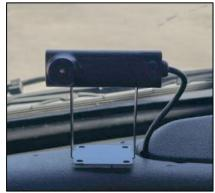
We offer a 3-inch mount to accommodate vehicles where steering wheel, seat adjusments and lower dashboards may create clearance issues for calibration.
