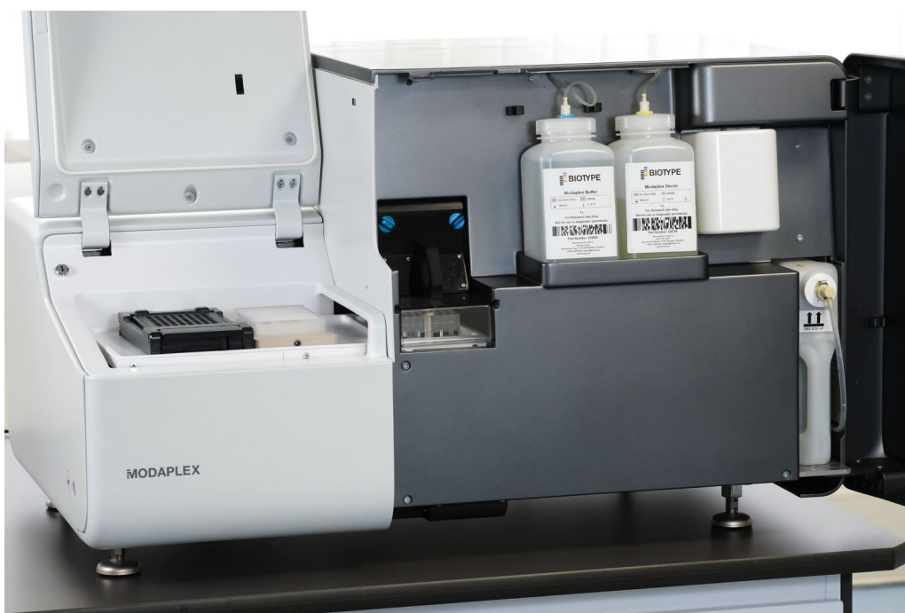
Figure 4: MODAPLEX instrument, view with sample door open (left) and consumables door open (right)
