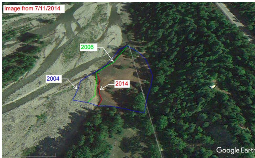
Figure 1: Approximate extent of tailings pile erosion into Lightning Creek over time based on past aerial photos (IDEQ, 2016).
