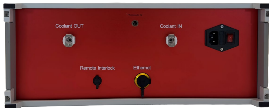
Figure 12 – Rear panel view of the 4U water-cooled chassis.
