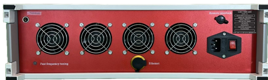
Figure 8. 770 nm fiber laser 3U chassis back panel air cooled.
