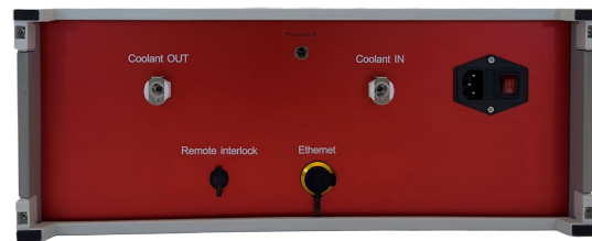
Figure 9. 556 nm fiber laser, 4U chassis back panel water cooled
