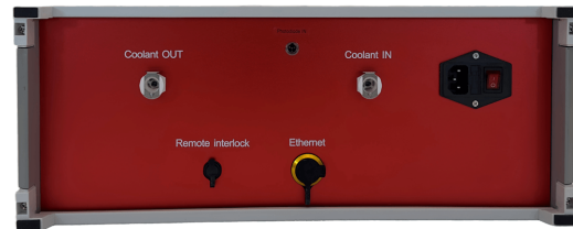
Figure 10 – 783 nm fiber laser 4U chassis back panel, water cooled.
