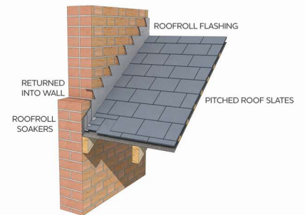
PARTY WALL SLATE ABUTMENT SIDE FLASHING
