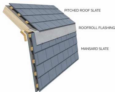
MANSARD SLATE ROOF DETAIL WITH FLASHING
