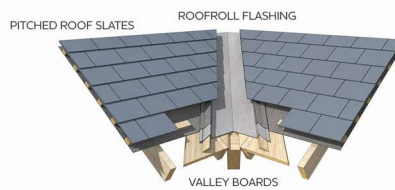
SLATE ROOF VALLEY DETAIL
