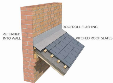
LEAN-TO SLATE ROOF ABUTMENT DETAIL
