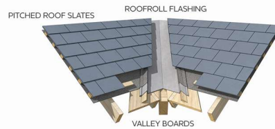
SLATE ROOF VALLEY DETAIL
