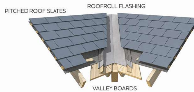
SLATE ROOF VALLEY DETAIL
