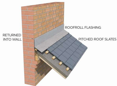
LEAN-TO SLATE ROOF ABUTMENT DETAIL
