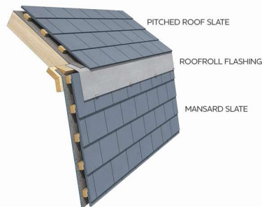
MANSARD SLATE ROOF DETAIL WITH FLASHING
