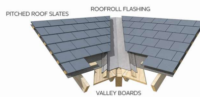
SLATE ROOF VALLEY DETAIL
