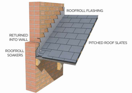
PARTY WALL SLATE ABUTMENT SIDE FLASHING
