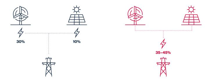
The figure shows that when WPP is connected alone, it uses its full reserved capacity for only 30% of the year, and PV only 10% of the year. However, if they connect together, they use the reserved capacity 35–45% of the time. In addition to saving network capacity, cable pooling also makes better use of it.
