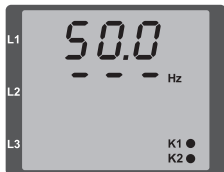
Fig. Rotary field direction can not be determined.
