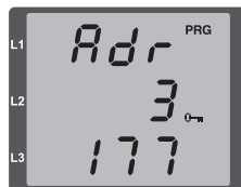
Fig. TCP / IP address, byte 3, value 177
