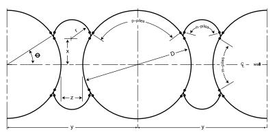
$\Theta$  is measured to the center of the 30° connection
