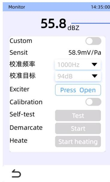
Sound Level Reading: Current data value measured by the noise sensor, including the weighting method display.
