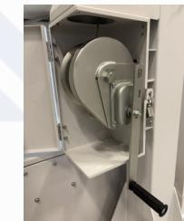
10. When the mast is fully raised insert pin to secure.
