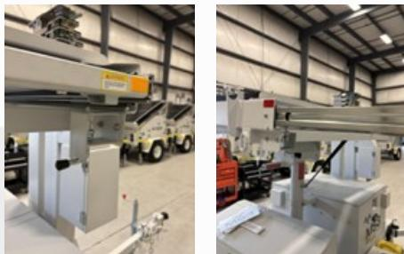
4. To rotate panels: Release pin at center post, Tilt panels to desired angle, engage pin to keep angle. Release pin at button of post, carefully swivel panels to face south, engage pin secure panels.
