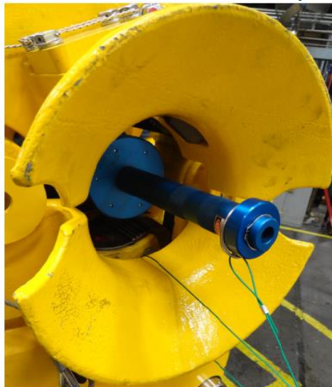
Figure 5 - Detail of the laser attached to the Top Drive shaft.
