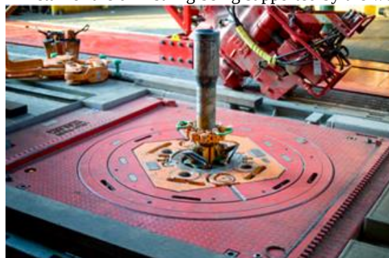
Figure 1 - Detail of the drill string being supported by the wedges
