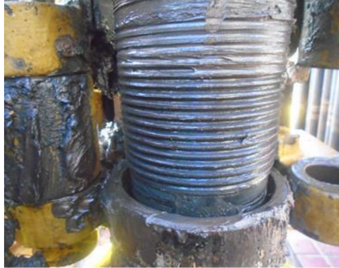
Figure 12 - Top Drive shaft aligned with drill pipe.
