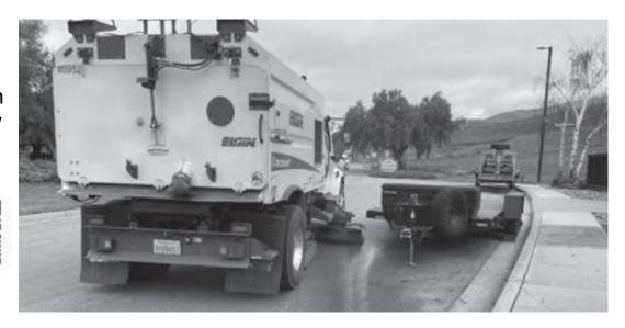
When vehicles and other obstructions block the street, sweepers cannot remove debris against the curb.
