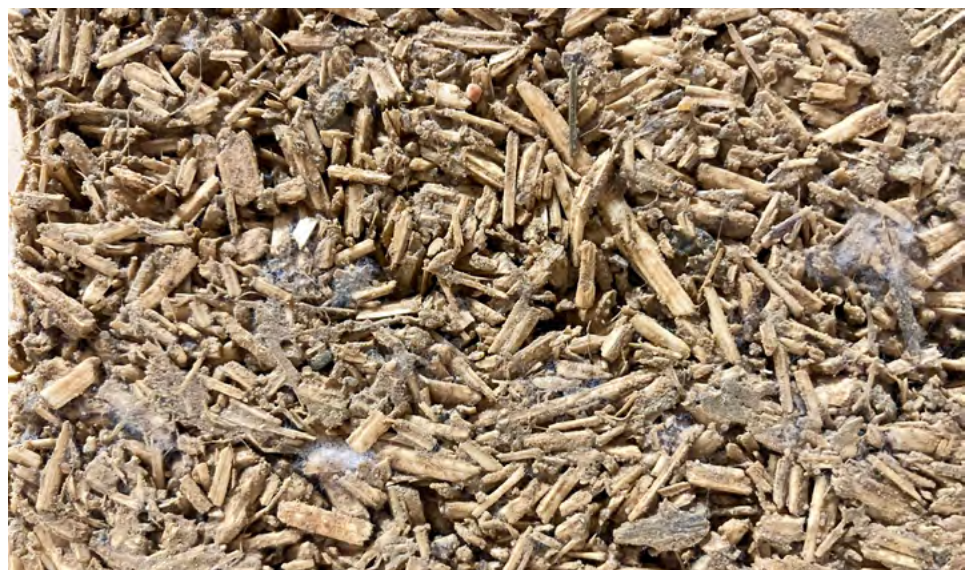
Figure 22. Mold on hemp-earth specimen with water to earth ratio 1:1. (Figure by author.)
