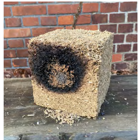
Figure 36. Fire resistance result - hemp lime (HL). (Image by author.)
