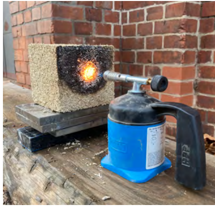
Figure 33. Fire resistance test - hemp lime (HL). (Image by author.)
