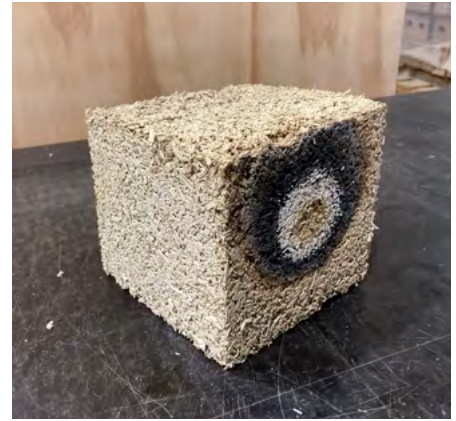
Figure 34. Fire resistance result - hemp lime (HL). (Image by author.)
