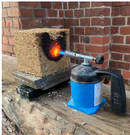
Figure 35. Fire resistance test - hemp lime (HL). (Image by author.)
