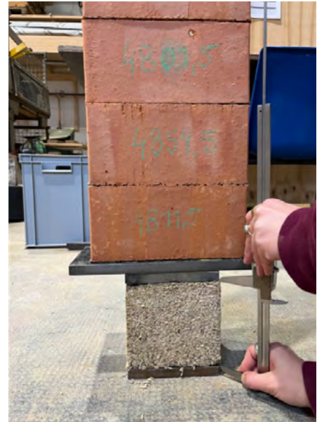
Figure 15. Monitoring deformation. (Image by author.)
