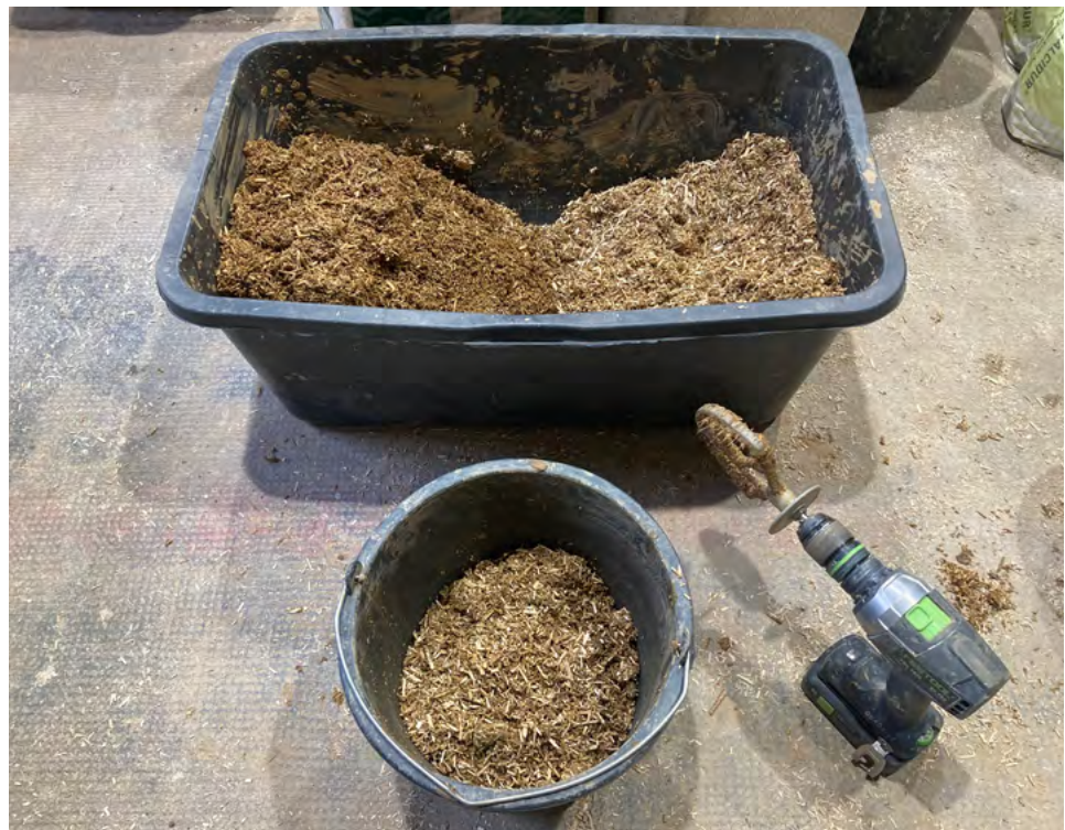
Figure 23. Mixing hemp-earth composite. (Image by author.)
