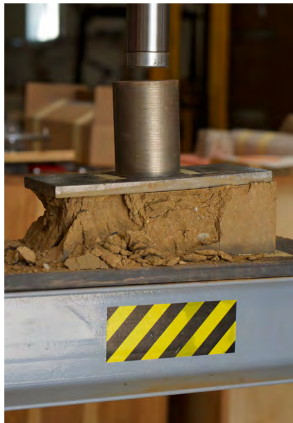
↑ → Earth Block testing © Tillmann Gebauer, 2025
