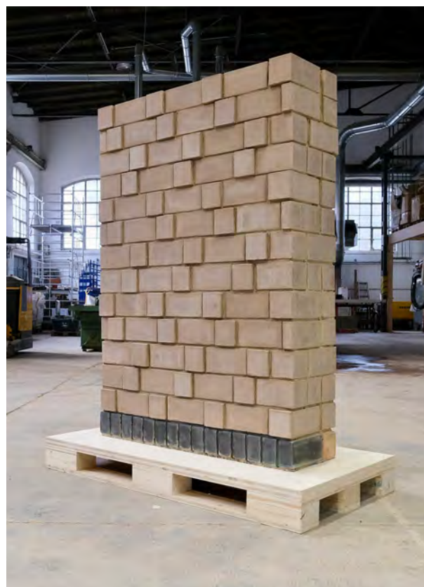
↑ Prototype of Earth Block Masonry for the HLH-Building → Development of a Timber-Earth Floor Plate (patent pending) © Bauhaus Earth, 2024f
