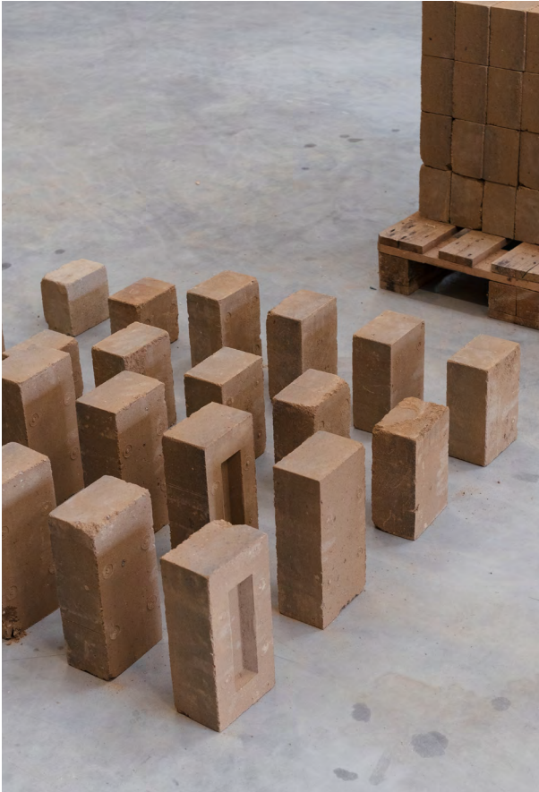
↑ Production of Compressed Earth Blocks © Florian Janowitz, 2025 ← Earth-Hemp-Blocks, Test Samples © Bauhaus Earth, 2024
