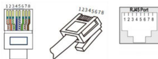
Figure 2-12 "Inverter CAN/RS485" port pins
