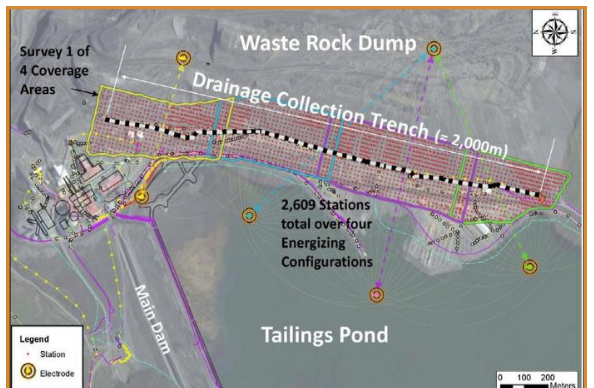
Survey 3 survey configuration with 908 measurement stations
