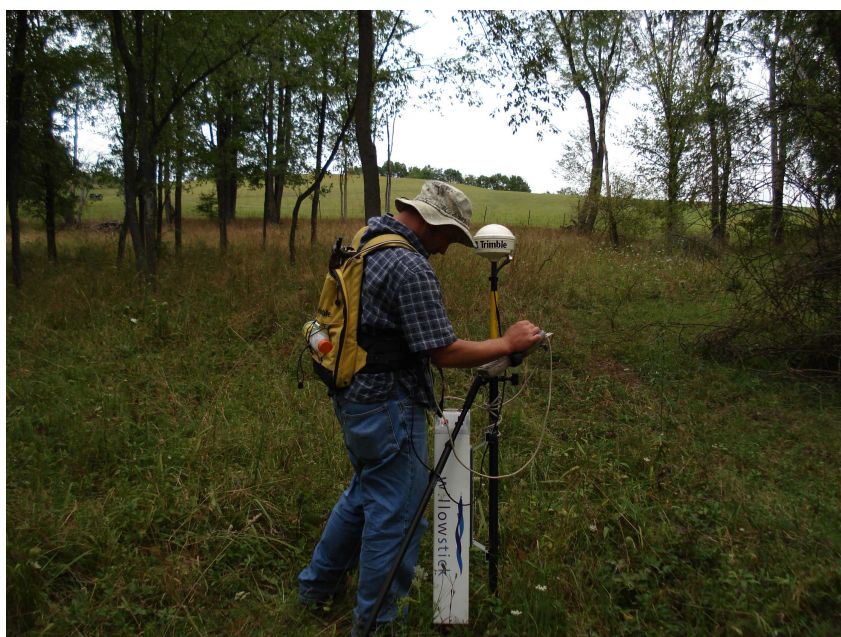
Figure 1 - Field Crew taking magnetic readings using CS-FDM equipment. GPS, Handheld computer, and data logger all shown.
