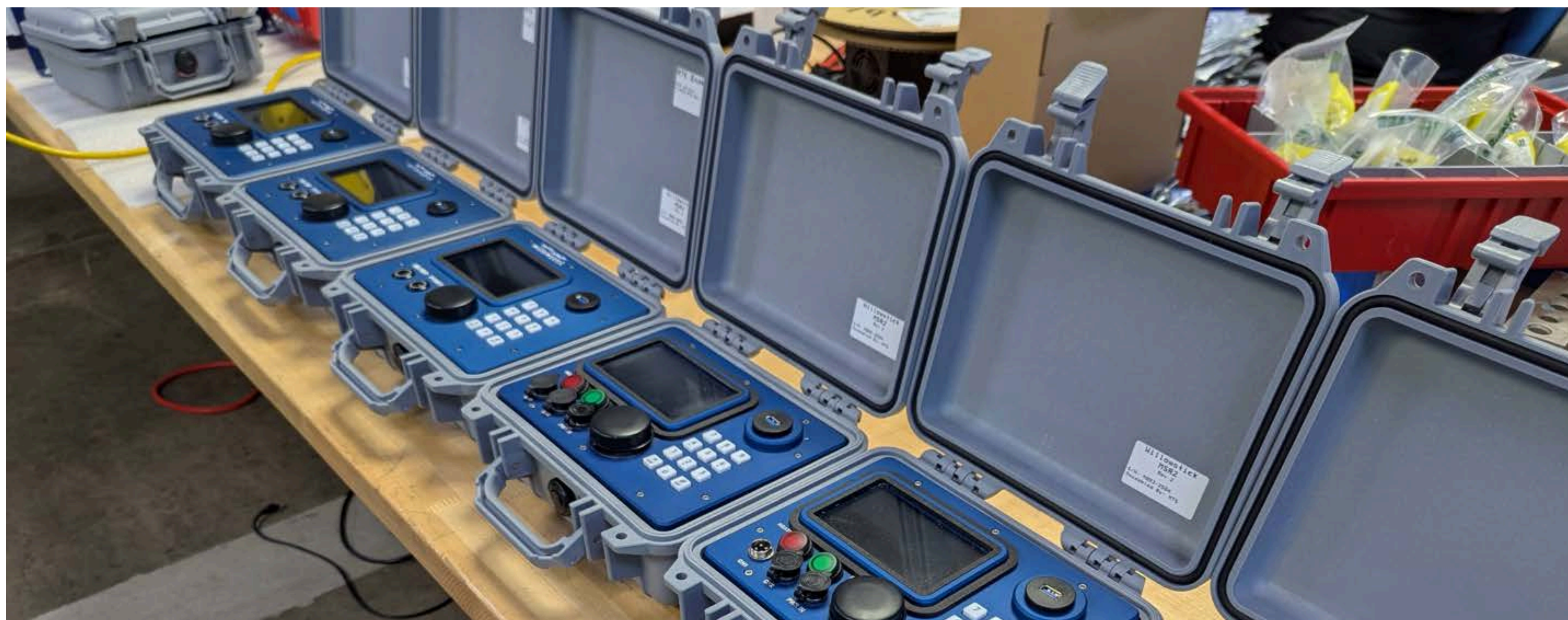
Figure 1 — MSR field instruments in pre-deployment staging. The MSR 2 instrument (current field-deployed version) is shown in its ruggedized carrying case, ready for field deployment. Multiple units are prepared for simultaneous multi-crew surveys.
