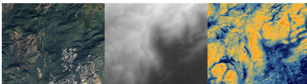
Figure 2 - In areas of high relief, and when acquisition off-nadir angle is high, orthorectification can lead to pixels and areas appearing stretched.
