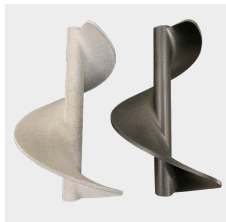
Grain Weevil robot augers printed with HP MJF using PA-12 material in natural gray (left) and with a black vapor polish finish (right).
