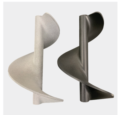
Grain Weevil robot augers printed with HP MJF using PA-12 material in natural gray (left) and with a black vapor polish finish (right).
