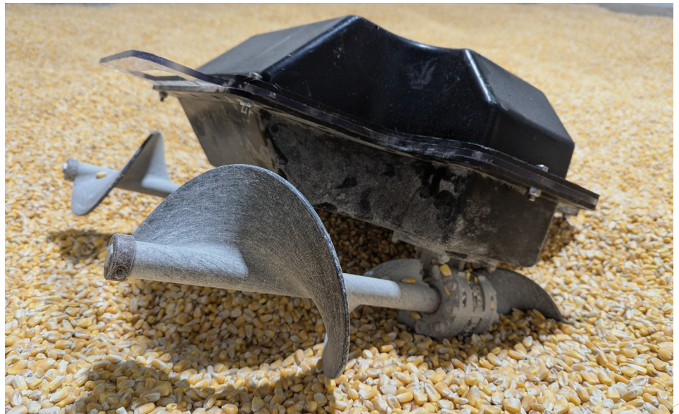
The Grain Weevil robot uses two sets of augers — one pair on the right of the robot and one pair on the left — to move through grain.
