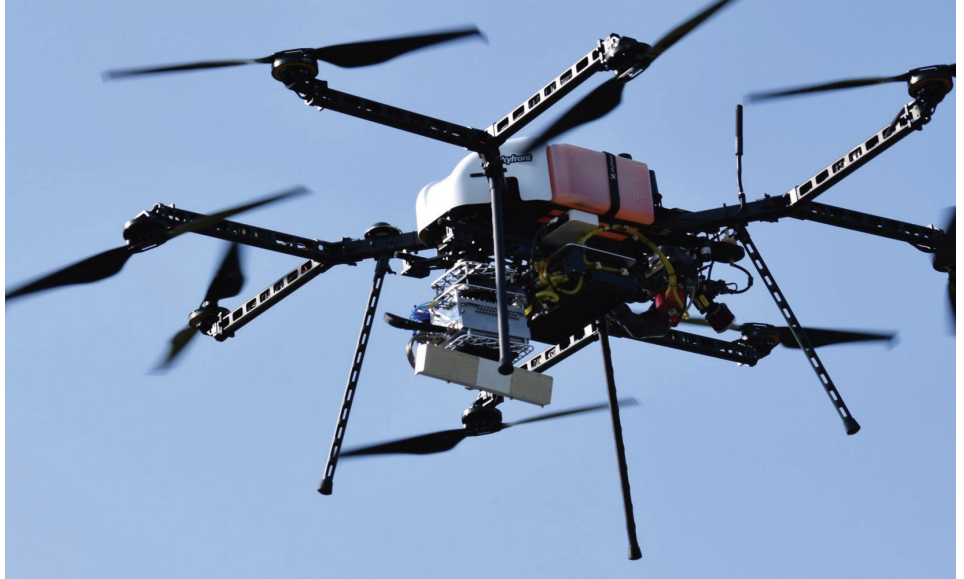
The Perimeter 8 hybrid drone stays airborne far longer than battery-powered models, thanks to the high energy density of gasoline.
