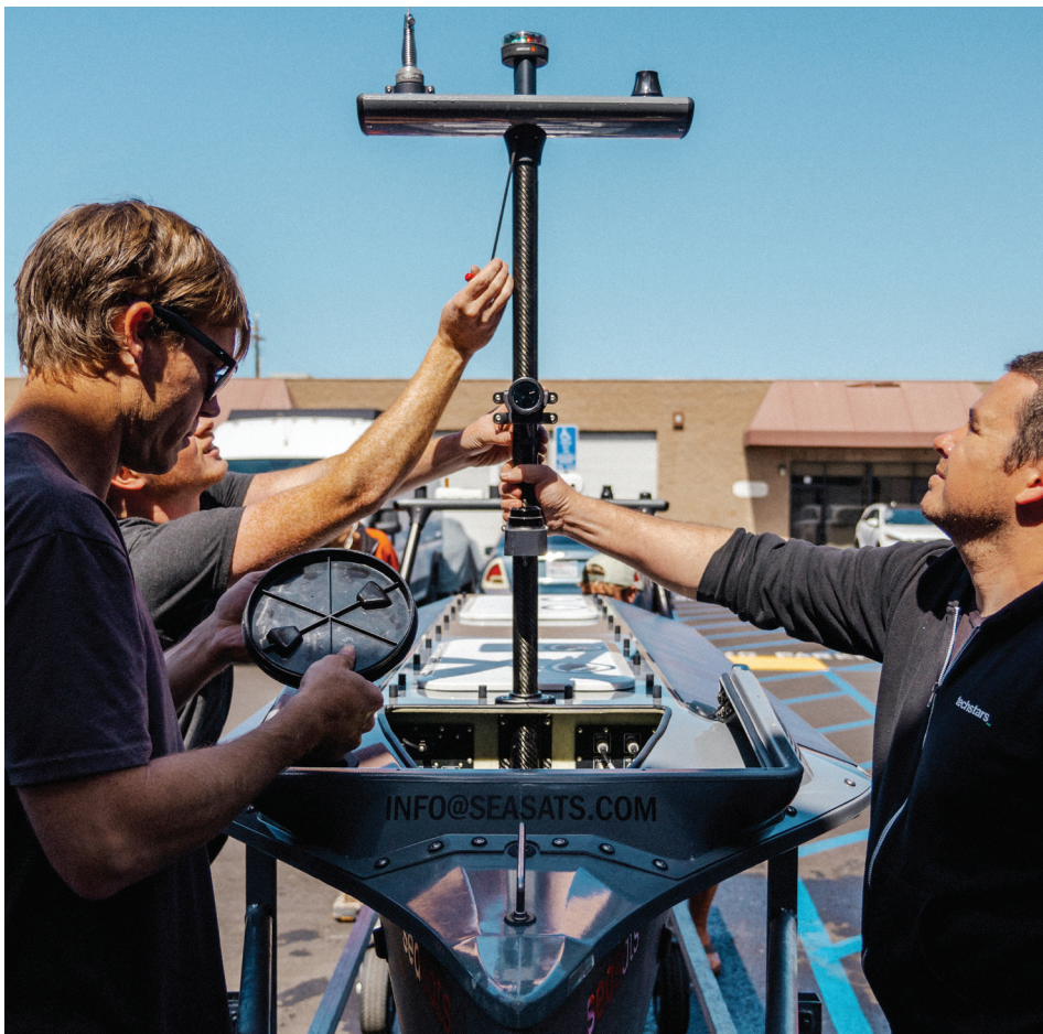
The Seasats team secures a 3D printed antenna to the bow of the Lightfish ASV.
