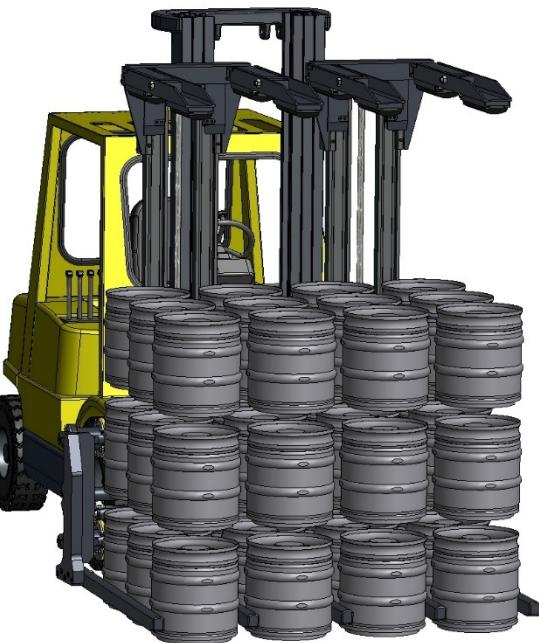
8. Lower the stabiliser onto the load.
