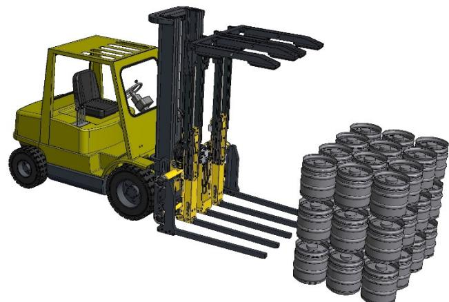
4. Open the clamp until the both sets of tines nicely clear the load.
