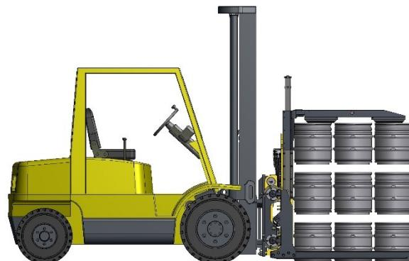
3. Raise the stabiliser clear of the load, observe clearance above it.
