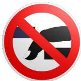
**Entrapment:** Finger trap decals are fitted to the unit where the risk of occurrence of trapping is conceivable. Always be aware that entrapment could happen in various locations on the attachment, always follow procedure and stand clear when in operation.
