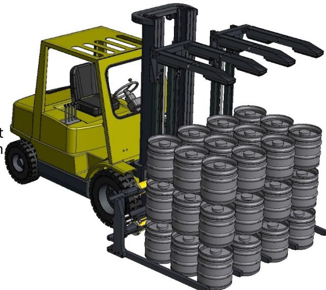
6. Raise the clamp until the tines are just below the rolling ring.
